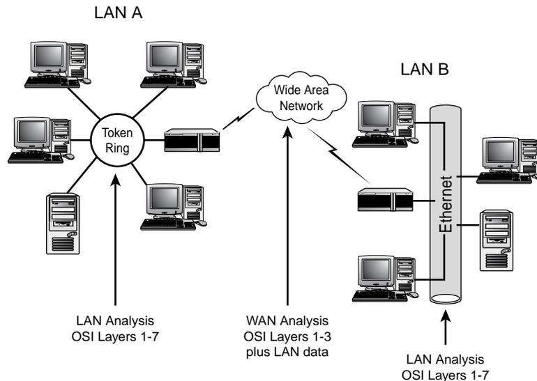
To properly diagnose a problem between a workstation on LAN A and a server on LAN B connected by the WAN, a LAN analyzer must decode those higher layers.
