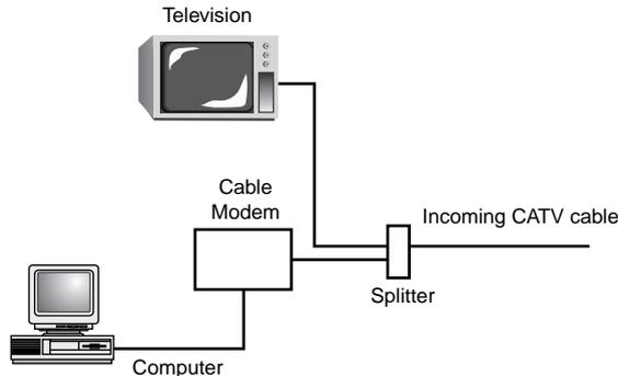
By taking advantage of the unused portion of the cable bandwidth as well as employing some interesting tricks of modulation, cable modems can supply users with access speeds at around 1Mbps. This is quite impressive in a home environment. Recent developments in software and operating systems allow multiple computers to take advantage of this single access point.
