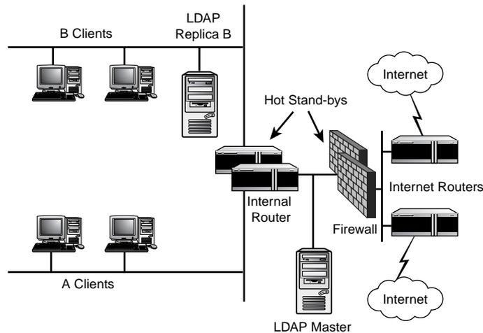
A more robust implementation is called *fault resilient*. Fault-resilient solutions generally use a fail-over type configuration but with care taken to ensure that redundancy within the device is as high as possible. An example of this would be two routers, each with dual power supplies, a UPS, and separate connections to the Internet.
