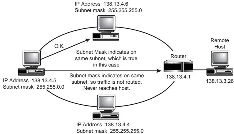
Figure 44.5 shows a subnet mask that masks too many bits. In this case, the subnet mask is 255.255.255.0. However, the network designers had intended the subnet mask to be 255.255.240.0, with four bits of the third octet used for the subnet and four bits as part of the host address.
