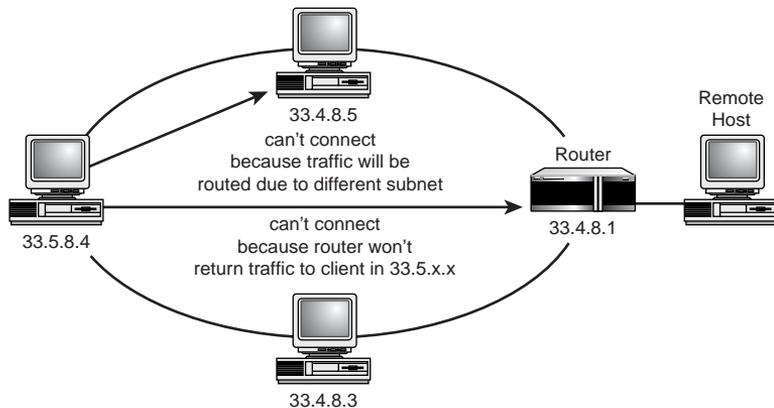
If a local client tries to send a message to 33.5.8.4, the message doesn't reach the client. If the local client uses the address as configured, the message is routed, which isn't the correct solution because the intended destination host is local. If the local client sends the message to what should have been the IP address, 33.5.8.4 doesn't receive the message because the IP address isn't configured correctly.
