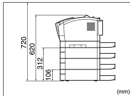
(Each rubber foot is 5 mm in height, and its tip is a square of 18 x 18 mm.)
