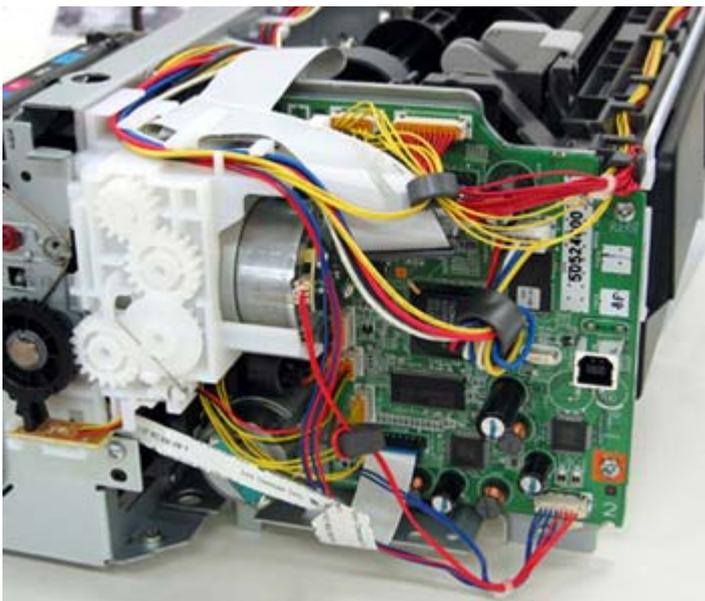
Logic board ass'y wiring (2 of 2).....Viewed from a different angle
