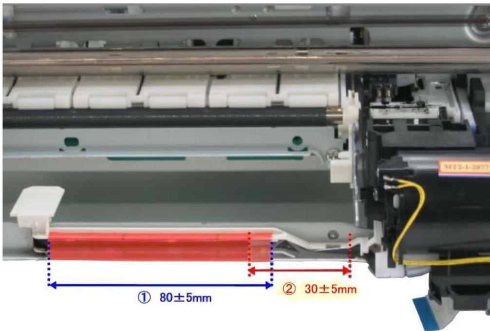
(II) After securing the waste ink tube with tape, be careful not to damage the tube in installing the printer unit chassis in the bottom case unit.
