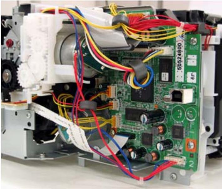
(II) Paper feed motor side wiring
