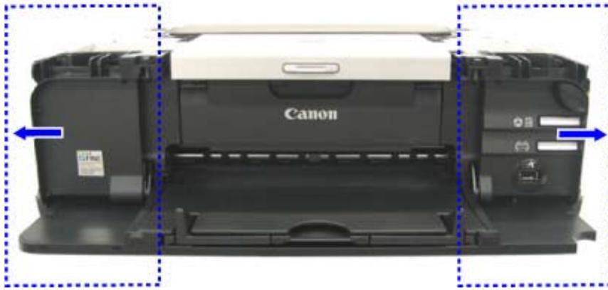
(IV) Hold the left and right corners indicated by the blue circle, and lift the upper case to remove it.
