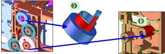
3) PR shaft / LF roller bushing
