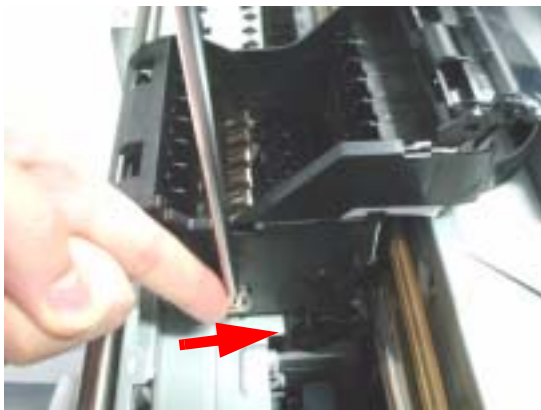
Figure 5-18. Head Fastener Fixing Method
