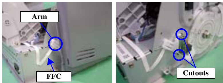
Figure 4-95. Reinstalling the PF Encoder Sensor
