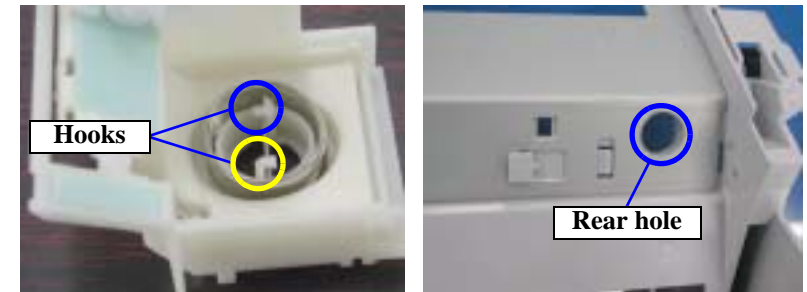
Figure 4-37. Installing the Compression Spring
