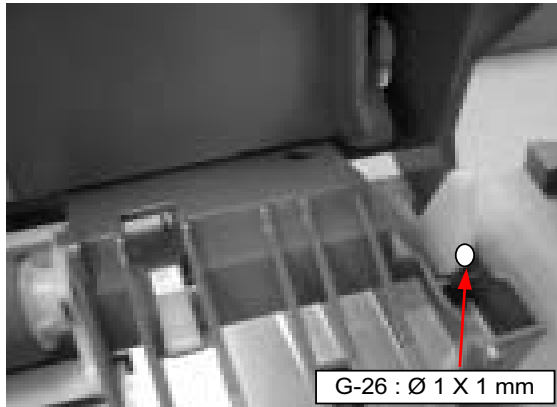
Figure 3-9. Lubrication point 6
