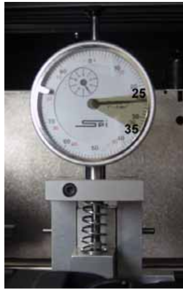
Figure 277: Gauge reading at correct X belt tension (Shading indicates acceptable range)
