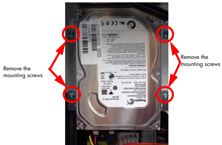
Figure 106: Hard drive mounting screw locations
