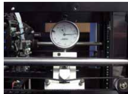
Dial Indicator position for Y-Drive belt tension check.
