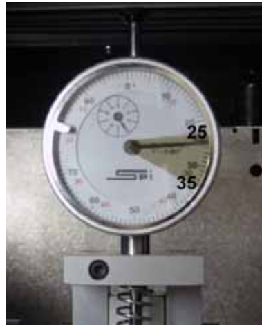
Figure 211: Gauge reading at correct X belt tension (Shading indicates acceptable range)
