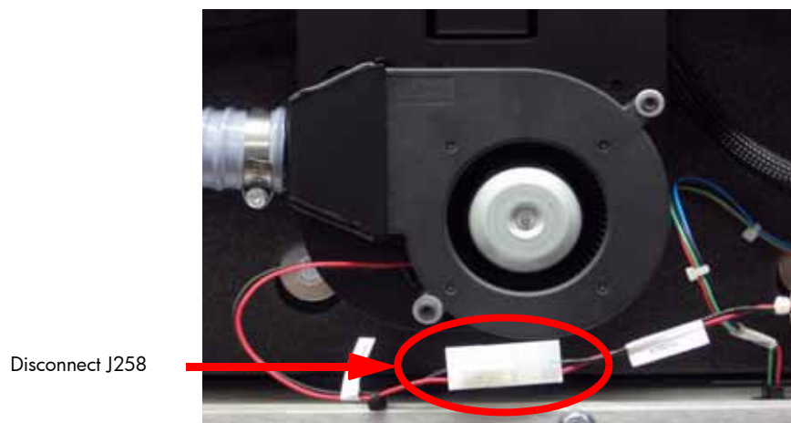
Figure 133: J258 cable location
