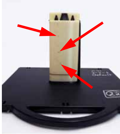
Example of embedded support
