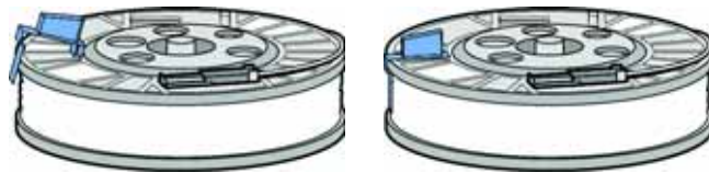
Figure 33: Installing material retaining clips
