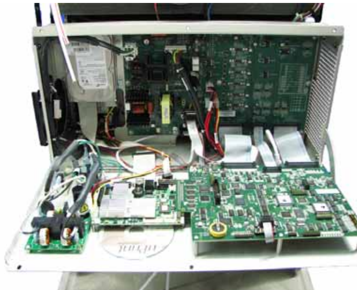
Figure 80: Electronics bay with cover lowered
