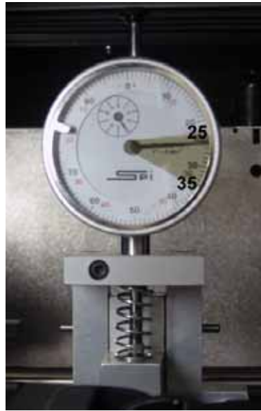
Figure 396: Gauge reading at correct X belt tension (Shading indicates acceptable range)
