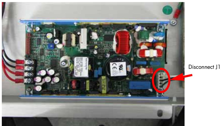
Figure 120: J1 cable location
