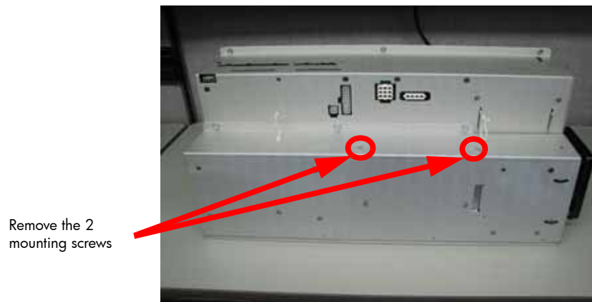
Figure 123: Removing the 2 mounting screws from the top of the panel
