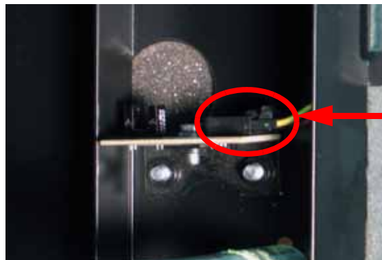
Figure 196: Y Home sensor cable location
