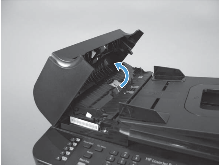
Figure 1-121 Remove the document feeder cover (1 of 3)
