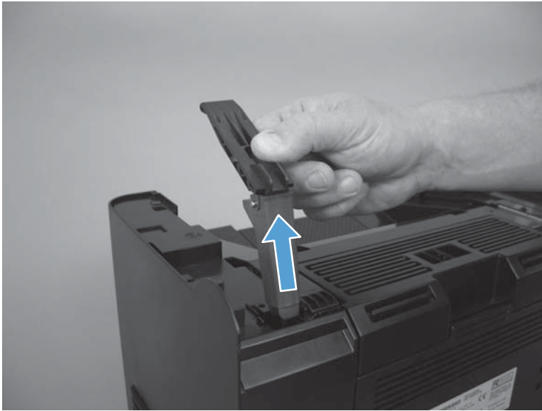
Figure 1-23 Remove the scanner hinges (2 of 2)
