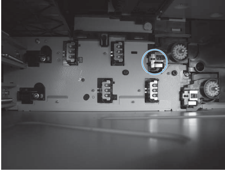
Figure 2-19 Tray 2 paper surface sensor
