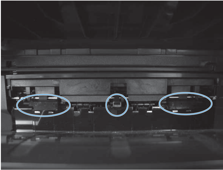
Figure 2-24 Output bin full sensor
