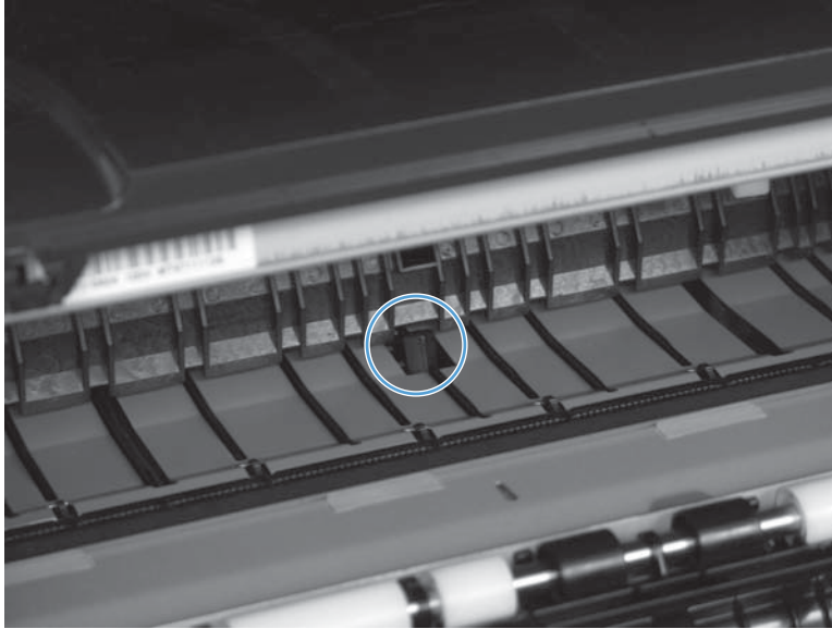
Figure 2-11 Fuser loop sensor
