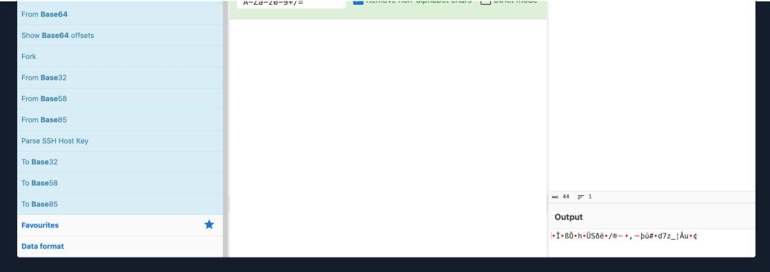
Then, we remove the From Base64 and select the AES Decrypt on the left side menu. Next, we configure the parameters with the key and the IV and give as an input the output we got from the From Base64,
