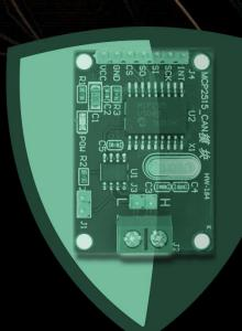
MCP2515 CAN Bus module support CAN protocol. It is used for sending and receiving CAN packets.
