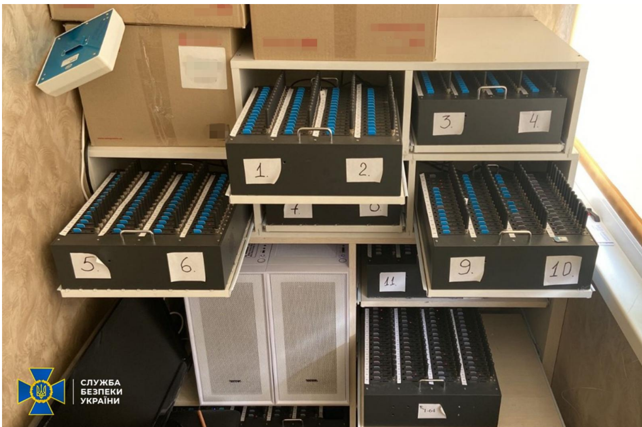
A Look Under the Hood: Here are terminals with SIM cards emulating unique and real human users in the virtual social world, this particular social botnet consisted of 100 sets of GSM gateways, over 10000 SIM cards, and laptops/computers for coordination and control. Distorting conflict situation and demoralising its adversary, it was recently captured by Ukraine post the Russian special military operation began in 2022 (Toulas, 2022).
