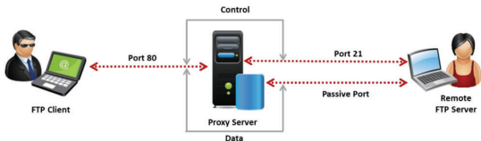
Figure 6.137: Schematic diagram displaying data communication between FTP server and FTP client
