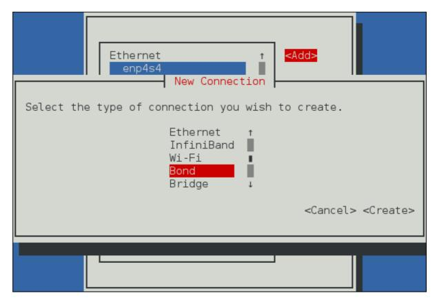
Figure 4.1. The NetworkManager Text User Interface Add a Bond Connection menu
