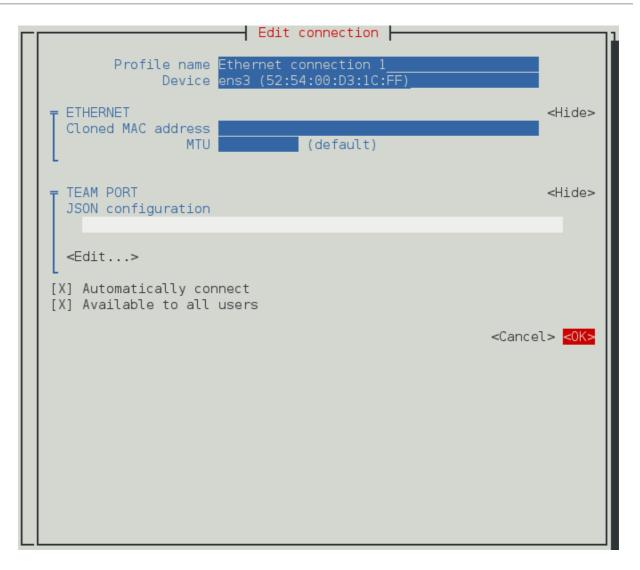
Figure 5.4. The NetworkManager Text User Interface Configuring a Team's Port Interface Connection menu
