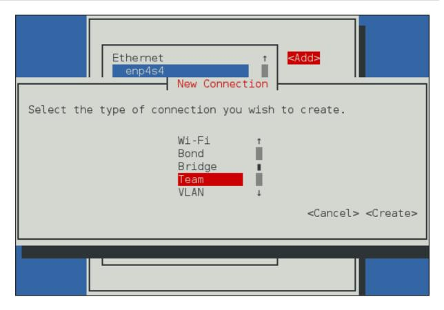
Figure 5.1. The NetworkManager Text User Interface Add a Team Connection menu
