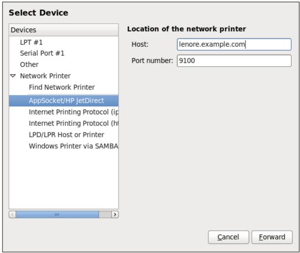
Figure 13.5. Adding a JetDirect printer
