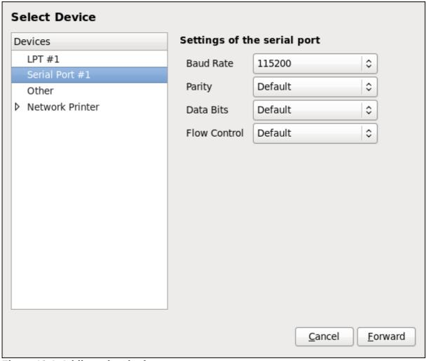
Figure 13.4. Adding a local printer
