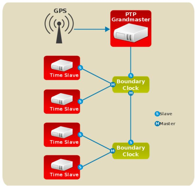
Figure 16.1. PTP grandmaster, boundary, and slave Clocks
