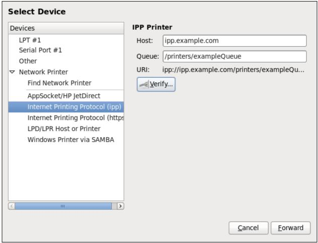
Figure 13.6. Adding an IPP printer
