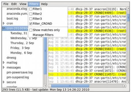
Figure 19.5. Log File Viewer - enabling a filter
