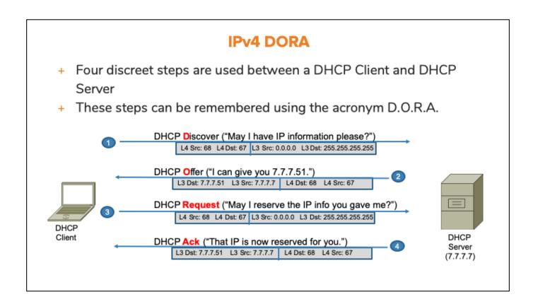
Notice that UDP port 68 is used to address (send things to) the DHCP Client...and UDP Port 67 is used to address (send things to) the DHCP Server.
