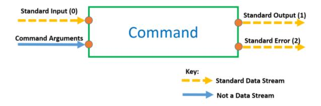
Standard Data Streams can be redirected and are identified using their stream number.
