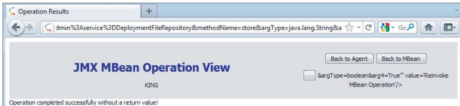
Figure 18-5: A successful attack using the JMX console to deploy a backdoor WAR file onto a JBoss server
