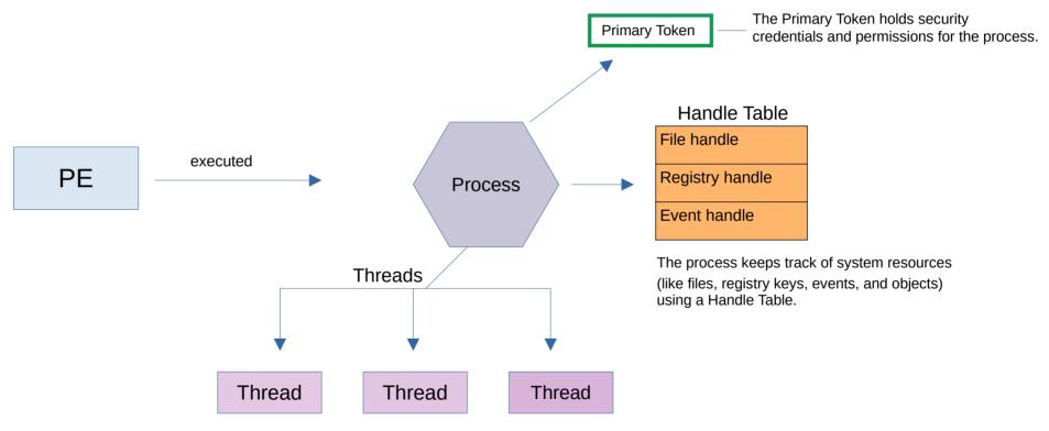
A process can have multiple Threads (units of execution).
