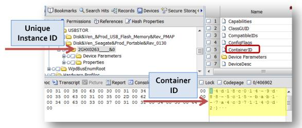
Figure 54 Container ID for Seagate Portable USB Device
