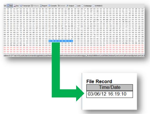
**Figure 26** This is the hex output of the stream. 106 bytes from the end of the stream is a group of 8 bytes, which are the date and time for this stream.
