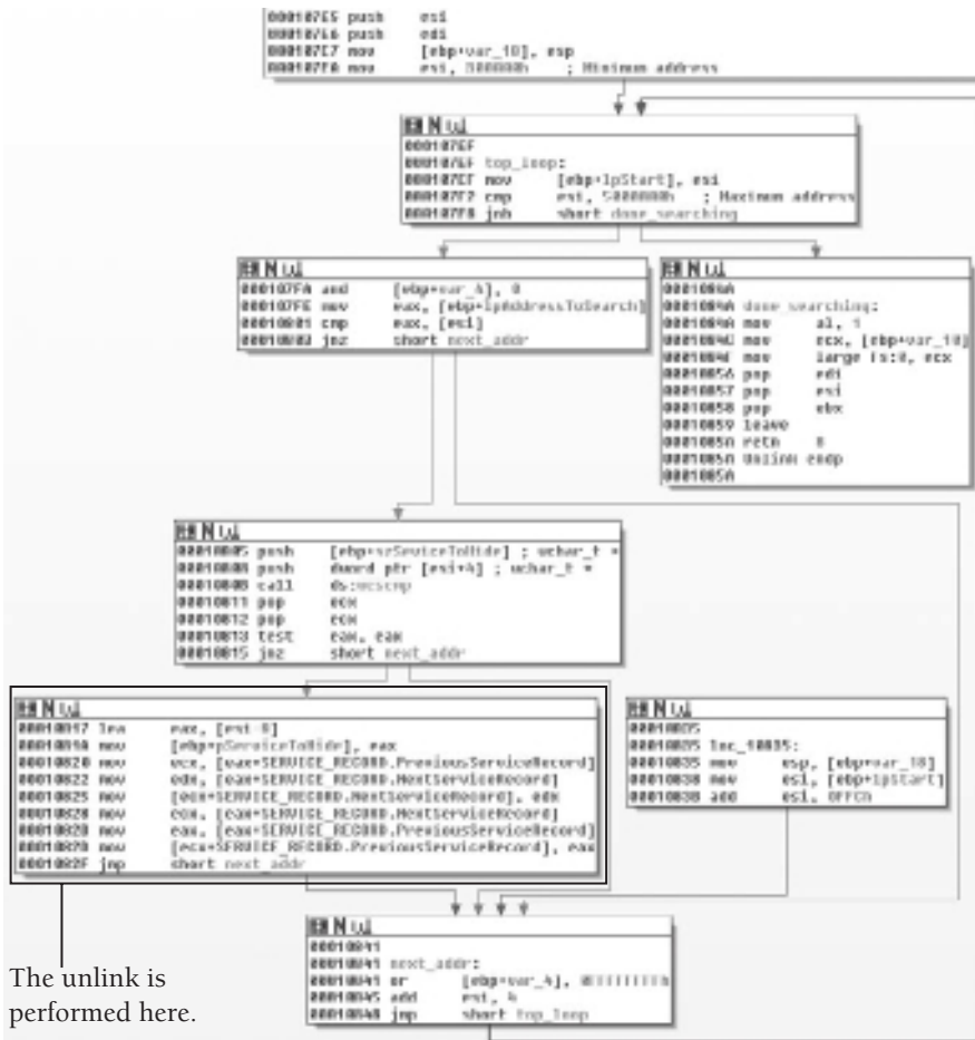
Figure 17-15: The Blazgel Trojan hides services by unlinking them.
