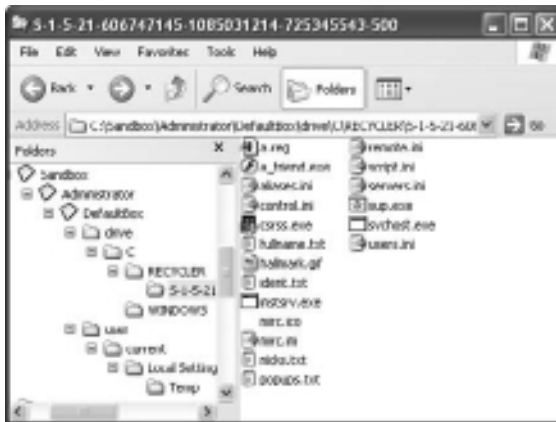
Figure 8-12: Sandboxie retains all files created during the malware's execution.
