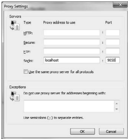
Figure 1-3: Internet Explorer Proxy Settings
