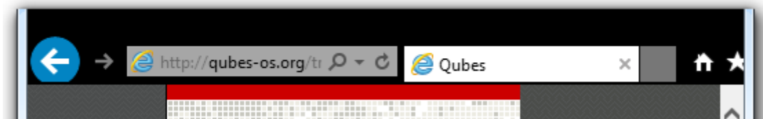
Fig. 7, Internet Explorer's title bar when the process doesn't have access to the Desktop Window Manager's ALPC API port
