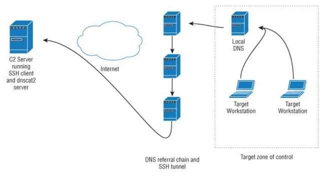
**Figure 3.1:** The beauty of this setup is that if your C2 is disrupted by security operations, you can point your DNS at another server.
