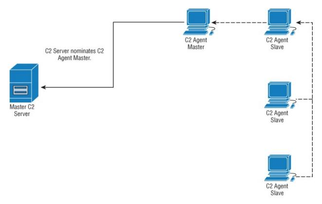
**Figure 8.2:** C2 uses Master for outbound connectivity.
