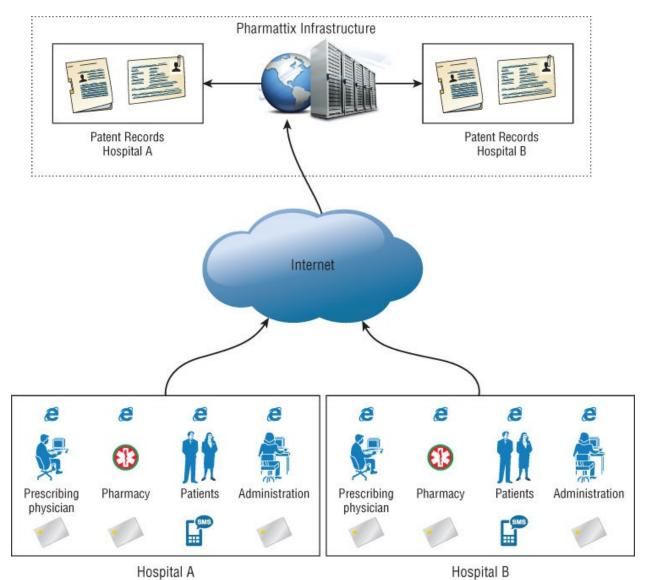
Figure 1.1: Pharmattix network flow
