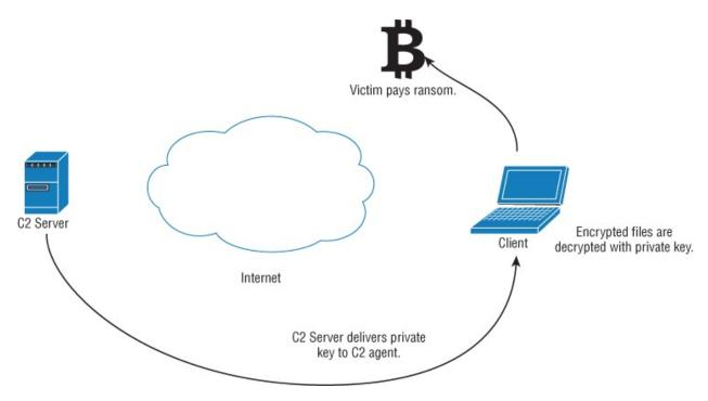
**Figure 5.4:** Decryption process flow.
