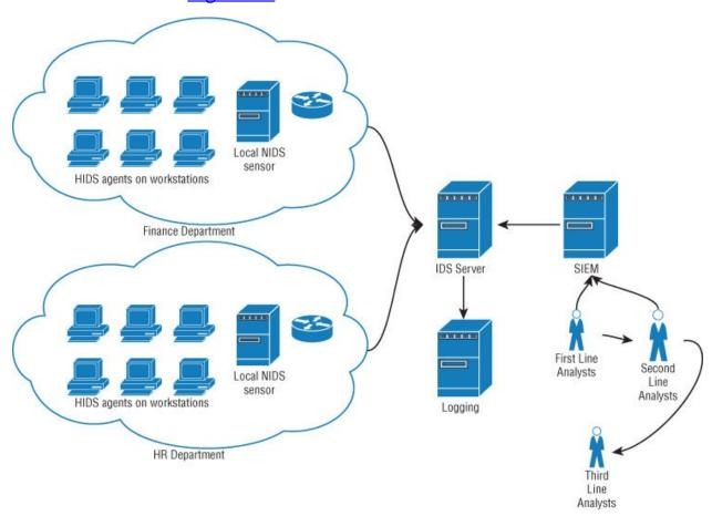
**Figure 3.2:** A basic intrusion monitoring setup.
