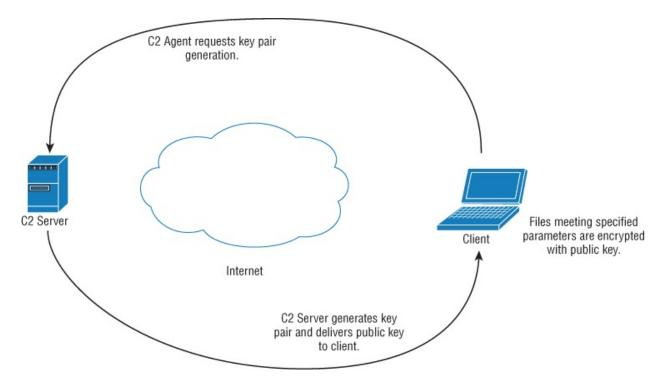
**Figure 5.3:** Encryption process flow.
