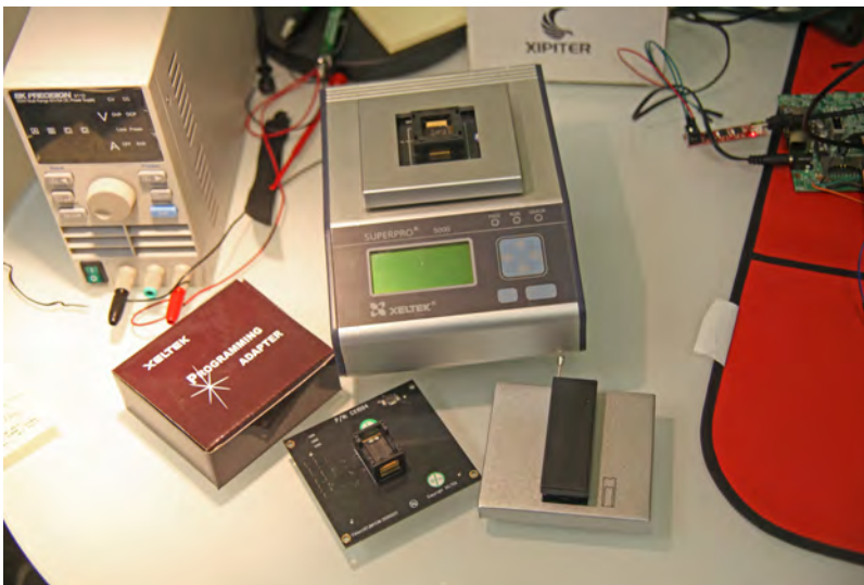
Figure 13-42: Xeltek SuperPro 5000E with adapters
