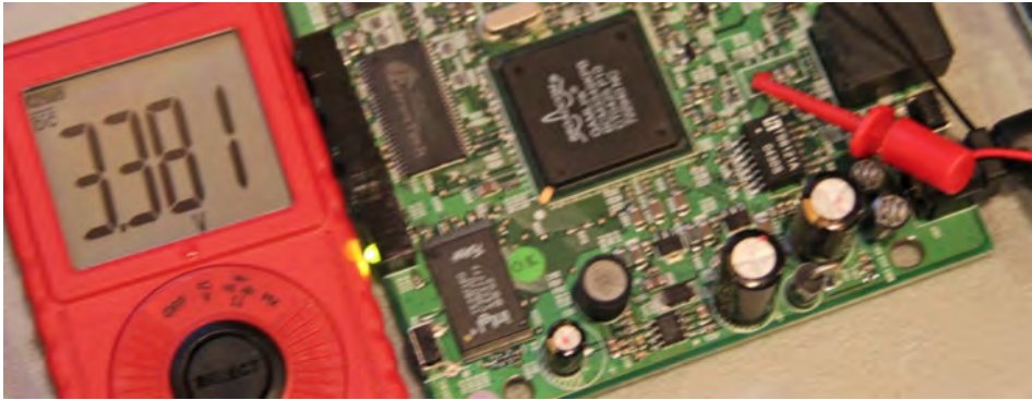
Figure 13-19: Broadcom BCM3349 voltage test
