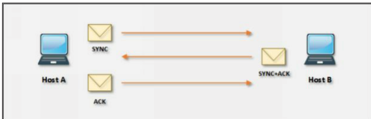
Figure 3-03 TCP Connection Handshaking
