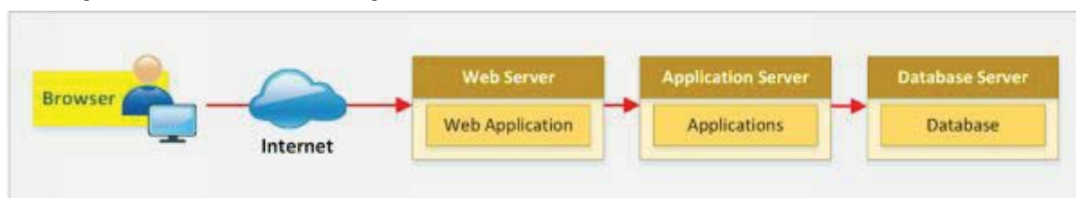
Figure 14-02 Web Application Architecture
