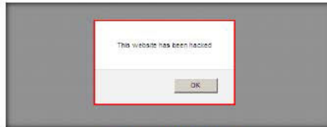
FIGURE 1.9: Cross Site scripting attack executed
