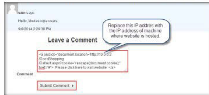
FIGURE 2.8: Entering the Stored XSS script in the vulnerable field
