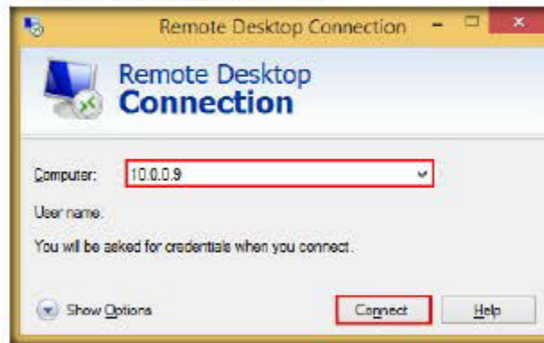
FIGURE 5.34: Establishing a Remote Desktop Connection
