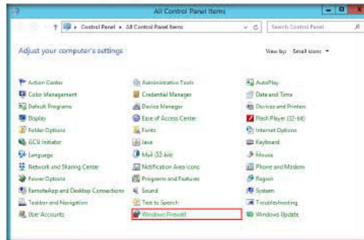
FIGURE 5.17: Opening Windows Firewall
