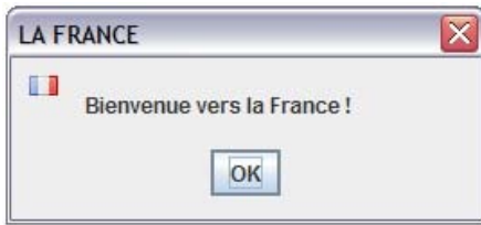
Figure 9–2. An almost completely localized dialog box displaying France-specific resources on Windows XP
