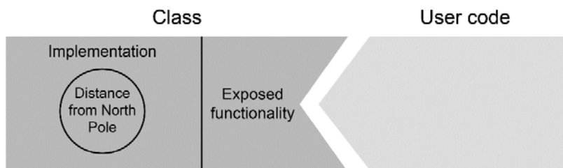
Figure 2.2: The implementation of the class changes, but since it is hidden from the user and the functionality was not changed, the user does not have to change how their code interacts with it
