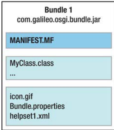
Figure 4-1. Components of an OSGi bundle
