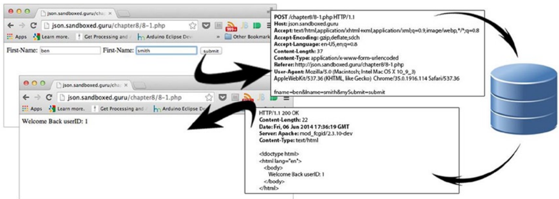
Figure 8-3. The full life cycle of an HTTP GET request
