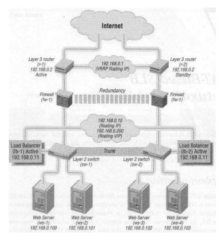
Figure 6-4. Flat-based SLB with a firewall
