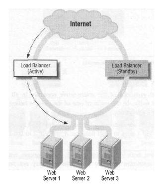
Figure 2-1, An active-standby redundancy scenario
