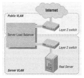
Figure 5-7. Two-armed SLB configuration
