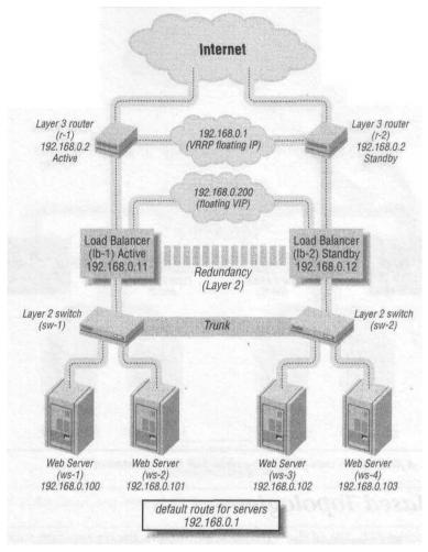
Figure C-3. Aflat-based, bridge-path, two-armed SLB implementation
