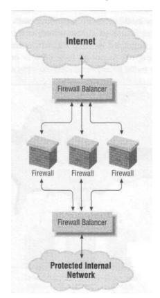
Figure 1-4. A common FWLB configuration
