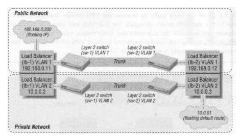
Figure 7-5. An incorrect redundancy scenario
