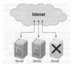
Figure 1-3- Afailure scenario with DNS-based load balancing
