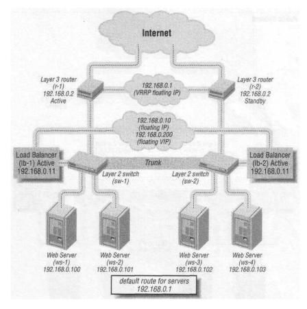
Figure C-5. A flat-based, one-armed DSR implementation
