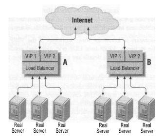
Figure 2-4. An active-active redundancy scenario variation
