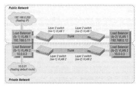
Figure 7-4. A correct redundancy scenario
