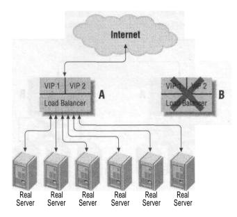
Figure 2-5. An active-active failure-recovery scenario
