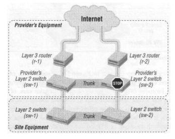
Figure 5-13. Sixpack with STP blocking
