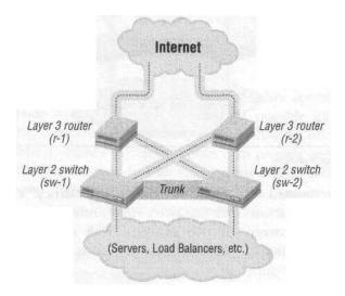
Figure 5-10. Four pack with cross-connects
