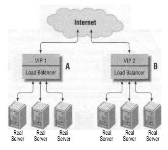
Figure 2-3. An active-active redundancy scenario
