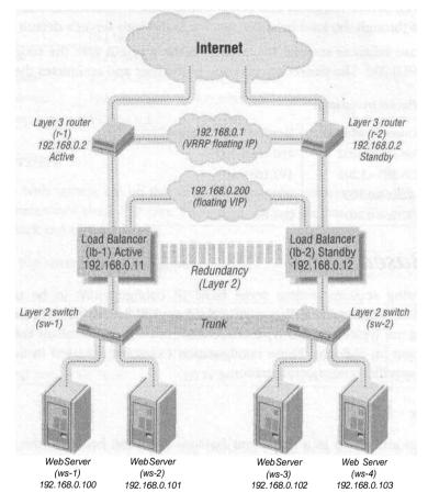
Figure 6-3. Flat-based, bridge-path, two-armed SLB
