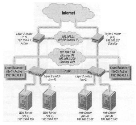
Figure C-4. Aflat-based, route-path, one-armed SLB implementation
