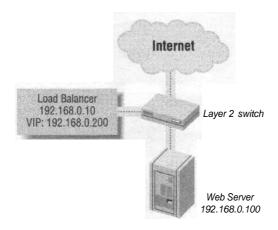
Figure 6-1. Simple, flat-based SLB
