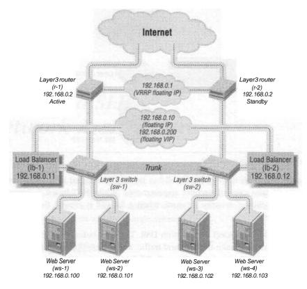
Figure 6-2. Flat-based, route-path, one-armed SLB
