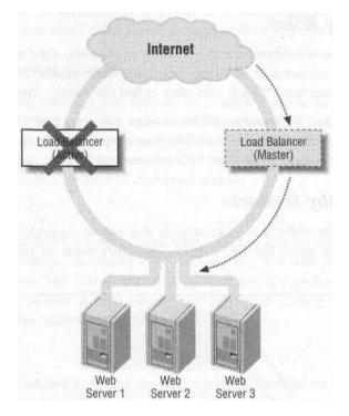
Figure 2-2. An active-standbyfailure scenario
