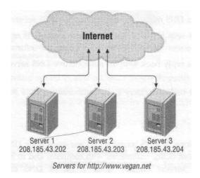
Figure 1-2. Traffic distribution by DNS-based load balancing
