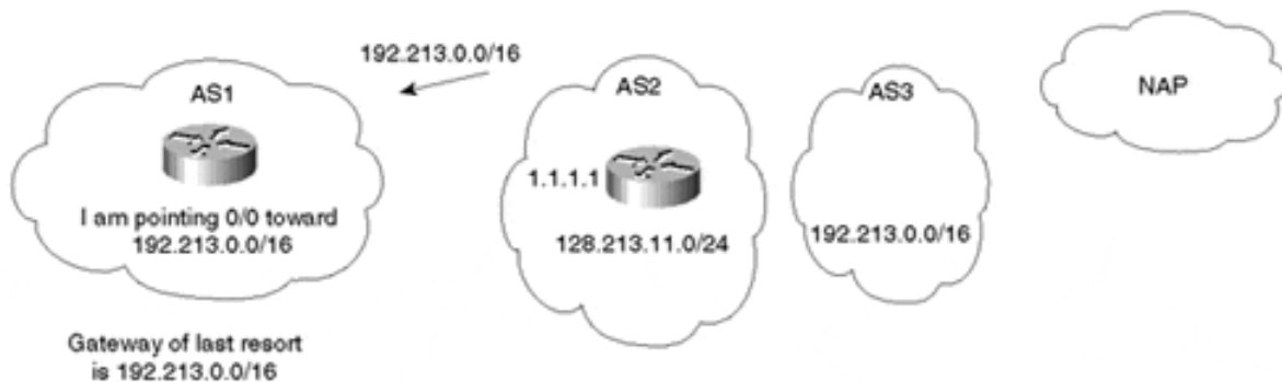
Figure 7-4. Pointing Default Toward a Network Number
