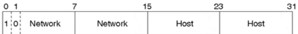
Figure 3-2. General Class B Address Format
