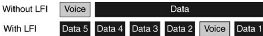
Figure 2-2. Link Fragmentation and Interleaving
