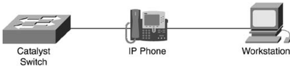
Figure 6-7. Cisco IP Phone Physical Network Diagram
