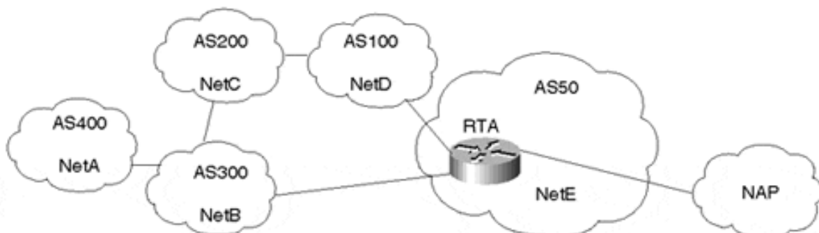
Figure 6-27. Sample Network Topology for Complex Regular Expression
