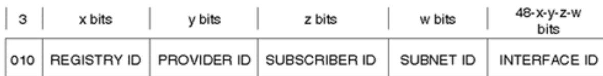
Figure 3-22. IPv6: Provider-Based Unicast Address Format
