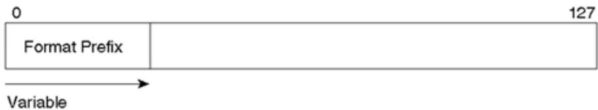
Figure 3-21. IPv6 Prefix and Address Format
