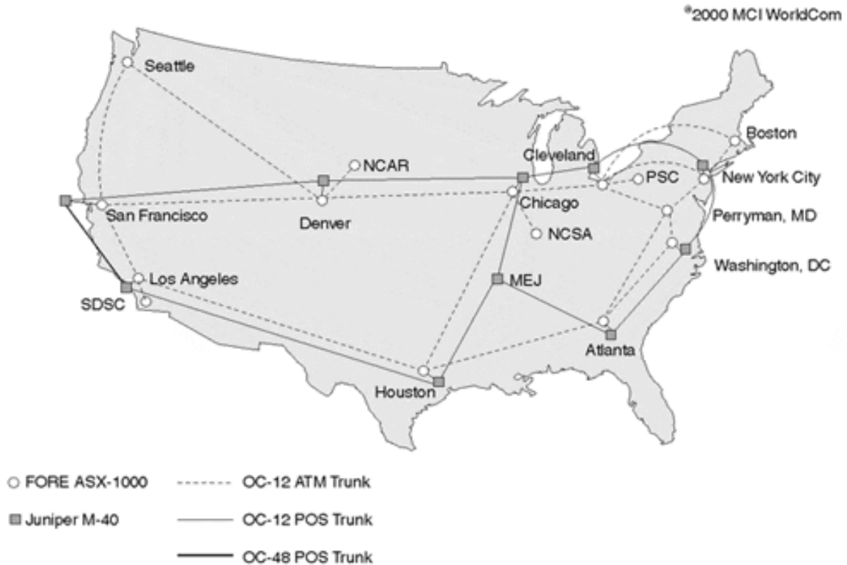
Figure 1-7. vBNS Backbone Network Map
