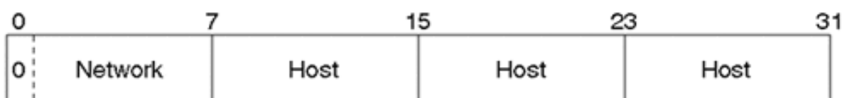
Figure 3-1. General Class A Address Format
