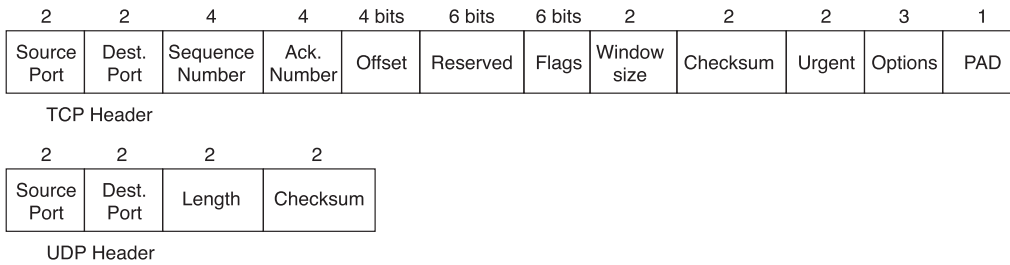
Figure 6-15 TCP and UDP Headers
