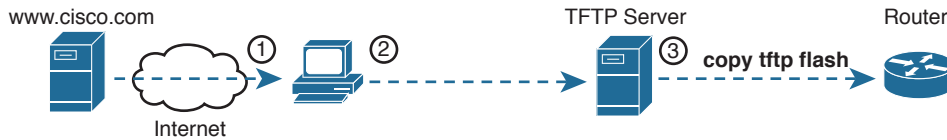
Figure 35-1 Copying IOS Image as Part of the Cisco IOS Software Upgrade Process
