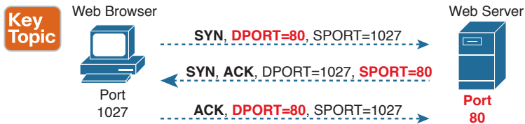
Figure 5-5 TCP Connection Establishment
