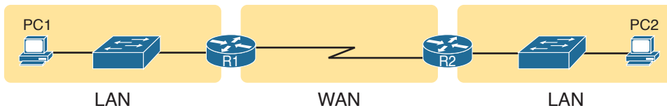
Figure 3-1 Small Enterprise Network with One Leased Line
