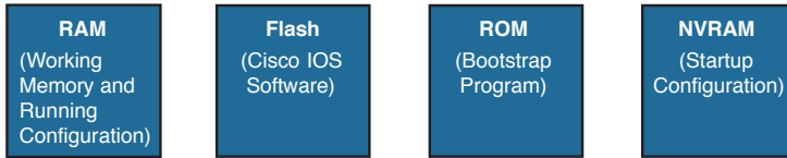
Figure 6-9 Cisco Switch Memory Types
