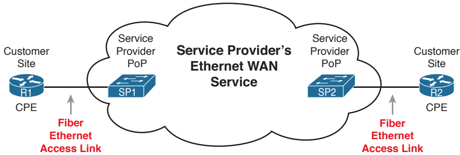
Figure 3-9 Fiber Ethernet Link to Connect a CPE Router to a Service Provider's WAN
