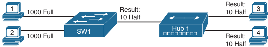
Figure 9-3 IEEE Autonegotiation with a LAN Hub
