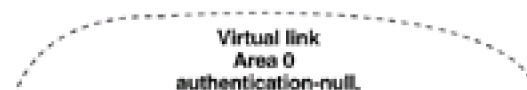
Figure 2-16. The Authentication Type Used on an OSPF Virtual Link Can Be Different from the Type Used in Area 0
