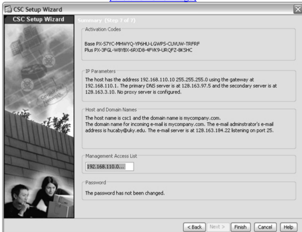
Figure 12-11. ASDM Updates the CSC with the Initial Configuration
