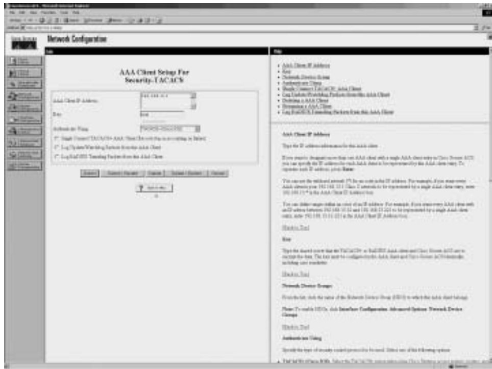
Figure 8-5 TACACS+ Network Configuration
