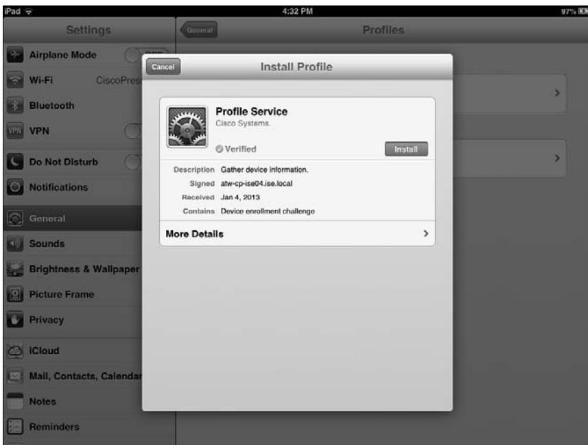
Figure 17-21 iOS: Install Profile
