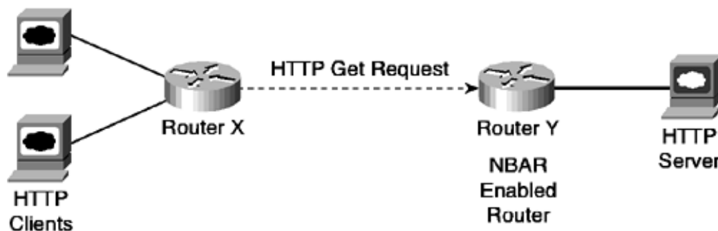
Figure 22-1. An NBAR-Enabled Router Classifying HTTP GET Requests Sent to an HTTP Server Behind It
