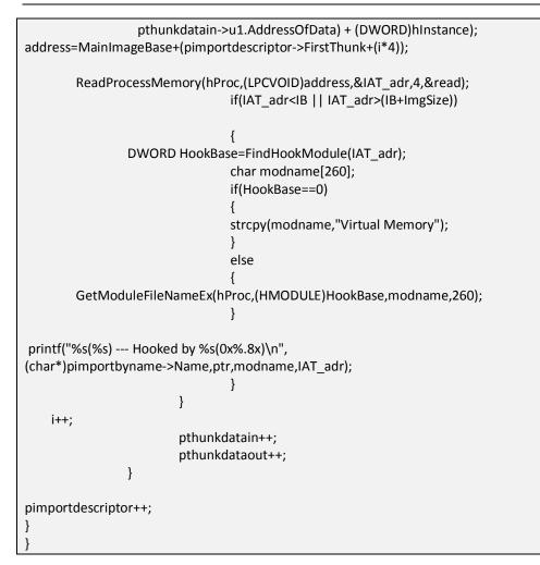
The IAT function uses two other functions. One finds a module address, and the other checks which library the address points to.
