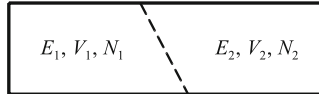
Fig. 10.1 A microcanonical ensemble divided into two parts, which corresponds to an isolated system divided into two subsystems
